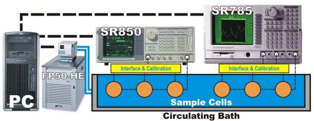
The SR785 dynamic signal analyzer also comes complete with a voltage source to excite the samples, however, it is designed to measure extremely fast, or transient, changes of the dielectric responses. Therefore, when the voltage is first applied to the samples, the SR785 will observe the fast "snap" that may occur to the protein, and the SR850 will observe the long-term changes-in-state as the voltage is
