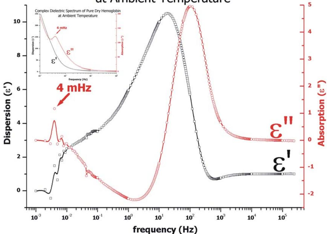
It must be emphasized that the 4 mHz response exhibits normal dispersion because the capacitive response is increasing with frequency, indicating a resonance effect. Usually, dielectric spectra are strictly observed as anomalous dispersion and the underlying mechanism involves relaxation processes.
